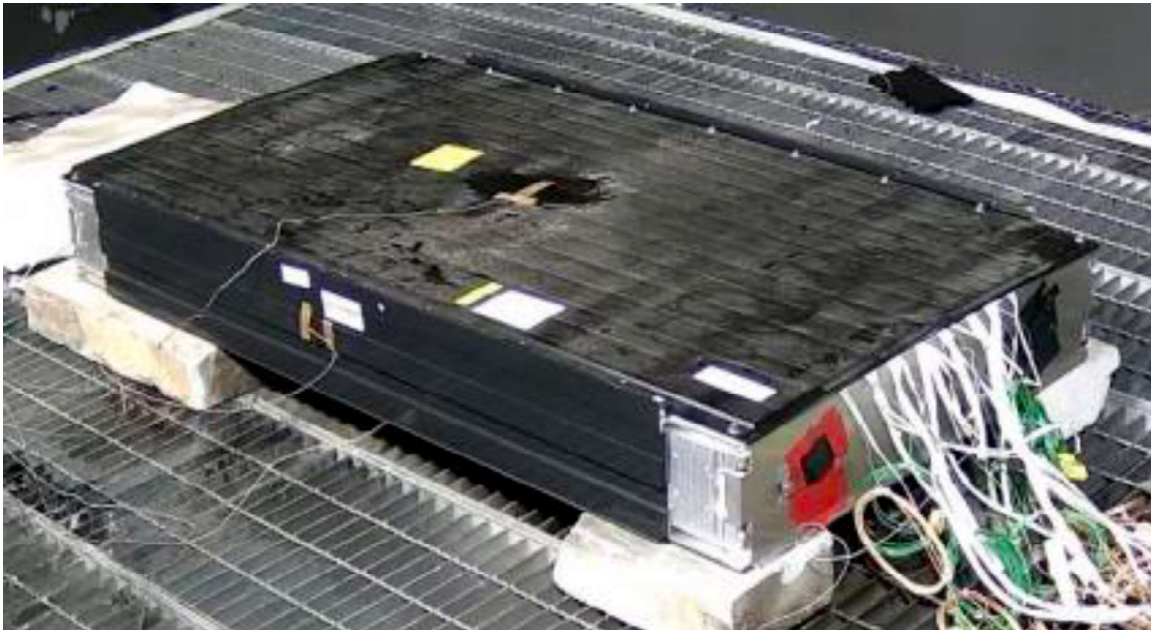
Figure 6 Tray tested to UL 9540A module level testing.
