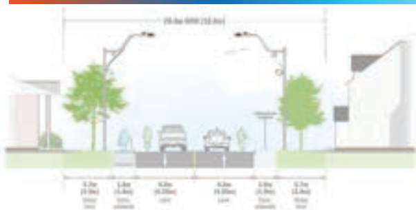
Local Street: 20.0m (66.0ft) Right-of-Way (Urban) Sidewalk on one side (both sides as required)
