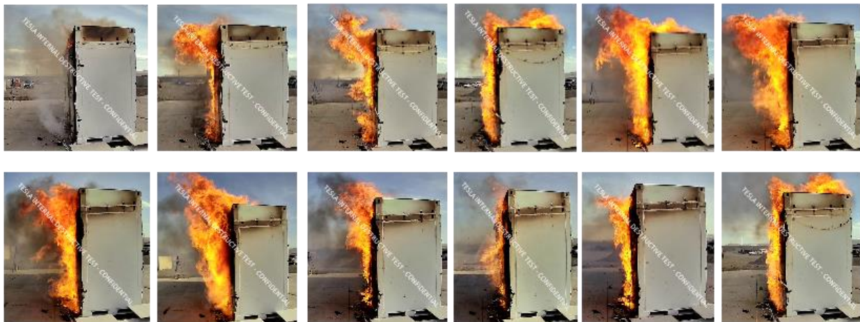
Figure 20 Fire progression during unit level destructive testing (first three hours): images captured every 15 minutes moving left to right. Initial flaming (top left), peak flame intensity occurring 60-90 minutes after initial flaming (top right) before diminishing for the remainder of the test (bottom left to right).
