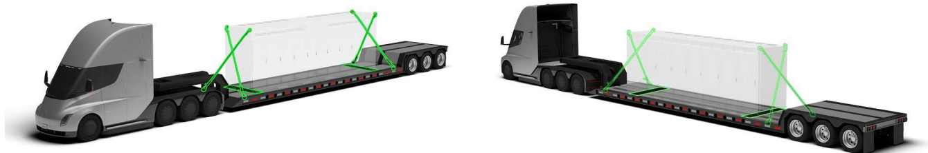
Figure 3. Preferred Securement System - Example - Chains and Friction Mat Locations Highlighted
